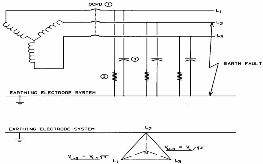
VOLTAGES TO EARTH OF AN IT-SYSTEM DURING A BOLTED FAULT TO EARTH CONDITION. WHEN A SOLID BOLTED FAULT OCCURS ON ONE PHASE THE PSEUDO NEUTRAL POINT IS DISPLACED AND THE VOLTAGE ON THE UNGROUNDED PHASES IS ELEVATED.
