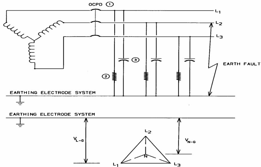
VOLTAGES TO EARTH OF AN IT-SYSTEM DURING AN ARCING FAULT TO EARTH CONDITION. AN ARCING FAULT TO EARTH IS POTENTIALLY MORE DESTRUCTIVE BECAUSE THE PSEUDO NEUTRAL POINT CAN BE OFFSET SIGNIFICANTLY FARTHER FROM THE GROUND PLAIN EACH TIME THE ARC RESTRIKES.
