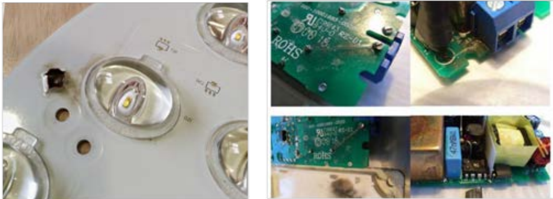
Examples of destruction to LED arrays and drivers due to lightning surges
