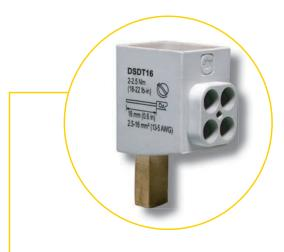
The DSDT16 is screw terminal dedicated to improve the wiring of DS surge protectors. This device allows an efficient and safe parallel connection («V» wiring) of a DS surge protector (SPD). «V» wiring is highly recommanded to avoid voltage drops in the parallel connection and to improve by this way the surge protection efficiency.
